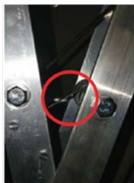
Location of Limit Switch on the arm
